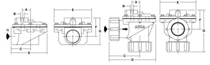
Fig. 1: Threaded pipe connection - aluminium
