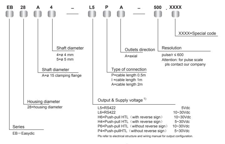
Only one channel allowed to be shorted-out if UB=5V, short-circuit to channel, 0V, or +UB is permitted if UB=10...30V, short-circuit to channel or 0V is permitted
