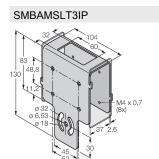
3073442 Protective housing with safety glas panel, for LT3 series
