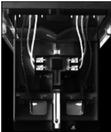
compulsory N/C contact safeguarded against contact
