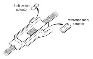
Reference mark and limit switch actuators can be mounted independently from each other, but within the limits specified by the relevant installation drawing.
