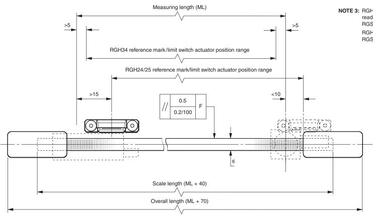
**NOTE 1:** The surface roughness of the axis guideway must be ≤3.2 μm. The parallelism of the scale surface to the axis guideway (readhead ride height variation) must be within 0.05 mm.
