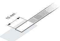
Mix up a sachet of glue (A-9531-0342) and apply a small amount to the underside of the end clamp.
