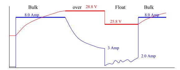
In the above graphic, the blue curve represents the amperage delivered to the battery in function of time. The red curve represents the voltage of the battery over time
