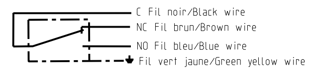
SCHEMA ELECTRIQUE (appareil au repos) DIAGRAM ELECTRICAL (switch at rest position)
